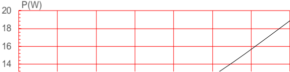
FIG.1: Maximum power dissipation versus RMS on-state current
