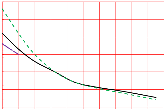
FIG.7: Relative variations of gate trigger current, holding current and latching current versus junction temperature
